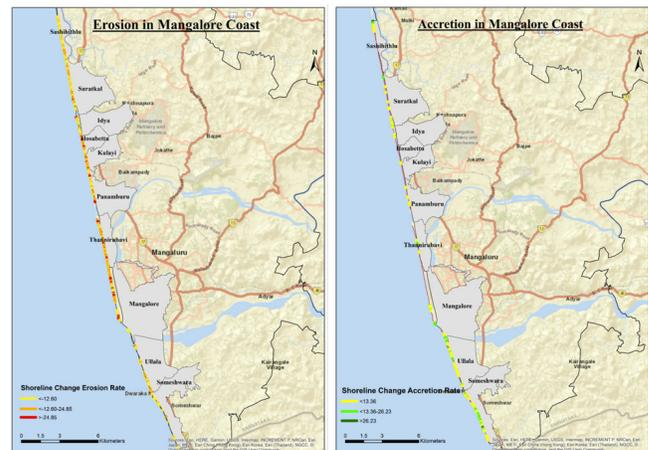
Figure 6: Erosion and accretion along the coast
