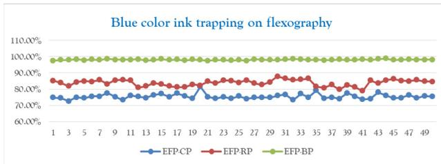
Figure 15: Blue color ink trapping for flexography printing
