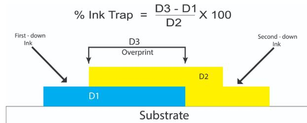
Figure 4: Ink trapping (Source: Chung & Hsu, 2008)
