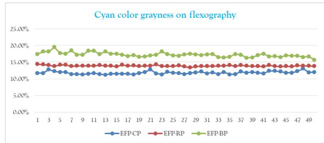
Figure 9: Grayness for cyan color for flexography printing
