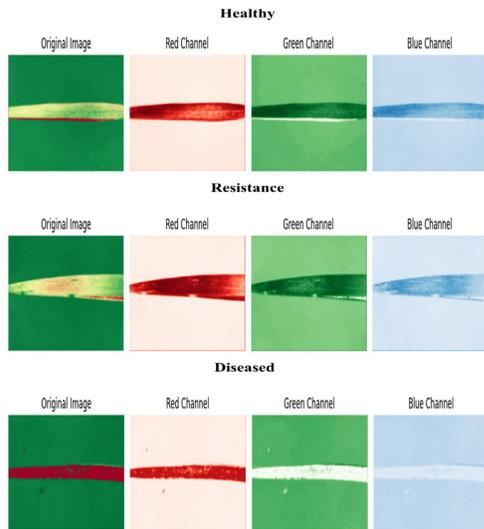
**Figure 1:** Separation of an image into its constituent color channels - Red, Green, and Blue (RGB)
