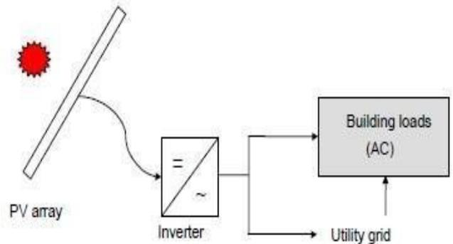
Figure 4: (b) Grid-connected PV system
