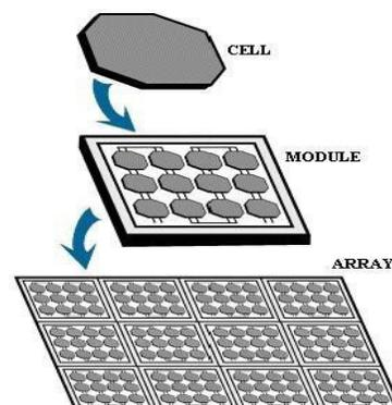
Figure 2: Photovoltaic module and array
