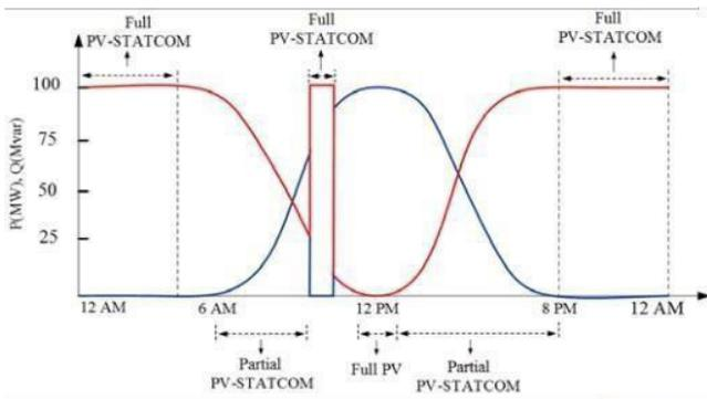
Figure 9: PV Real and Reactive power during 24 hours on a sunny day
