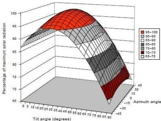
Figure 3: Variation of annual sunlight levels as a function of tilt and azimuth angles.
