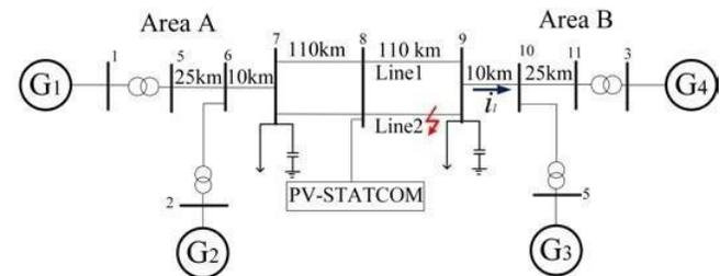
Figure 11: Single-line diagram of a Two-Area system with 100 MW PV plant connected to midline 12 Bus FACTS power system
