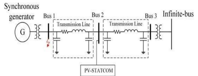
Figure 10: Single-line diagram of a SMIB system with a 100 MW PV plant connected to a midline Two-Area Four Machine System:
