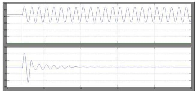
Figure 17: Nighttime (a) Midline real power without POD with PV STATCOM control, (b) PV- STATCOM reactive power during POD
