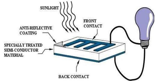
Figure 1: Conversion of light energy to electricity by using solar cell
