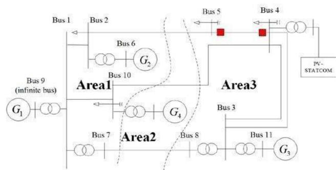
Figure 12: 12 bus FACTS power system with 100 MW PV solar systems at bus 4
