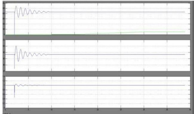
Figure 15: (a) Midline and PV system real powers, (b) PV-STATCOM reactive power, (c) Midline voltage during POD and normal ramped power restoration
