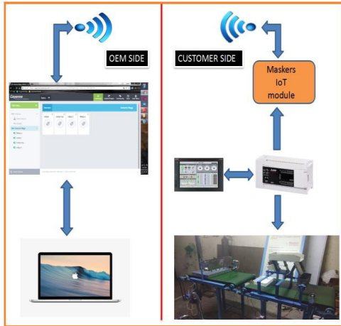
Figure 1: Block diagram of Virtual control of industrial machinerie for smart manufacturers
