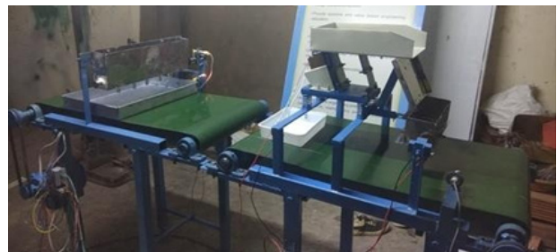
Figure 6: Conveyor system of proposed machine
