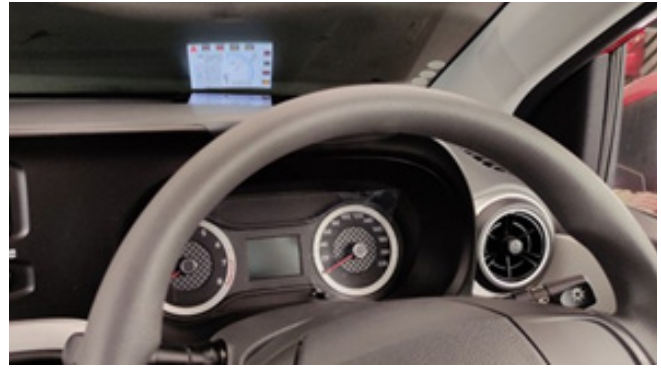
Figure 12: Experimental setup with Mobile phone as the projector
