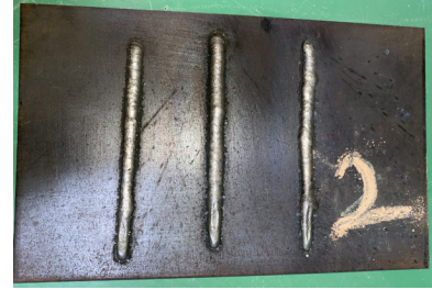
Figure 16: Hardfacing trials 4,5 and 6
