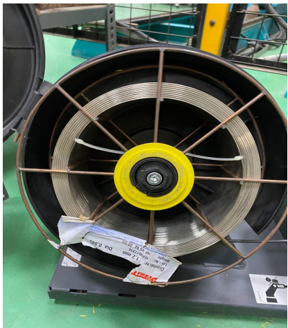
Figure 1: 1.2 mm Diameter Stellite 21 Filler
