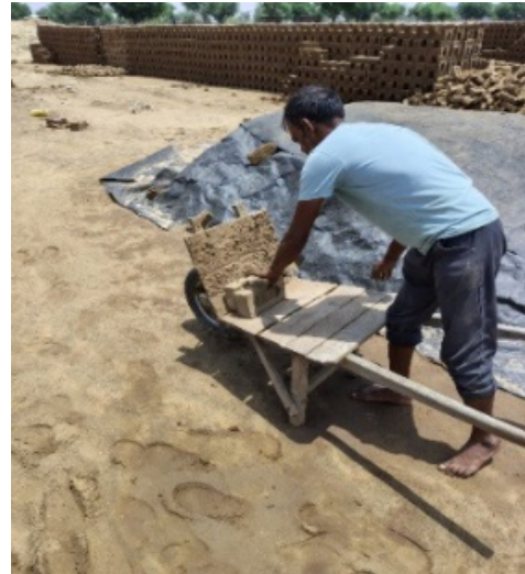
Figure 3: Moulding (Bharai) Process
