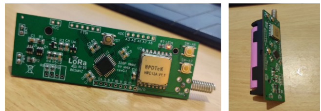
Figure 6: An upgraded and miniaturized water sensing node
