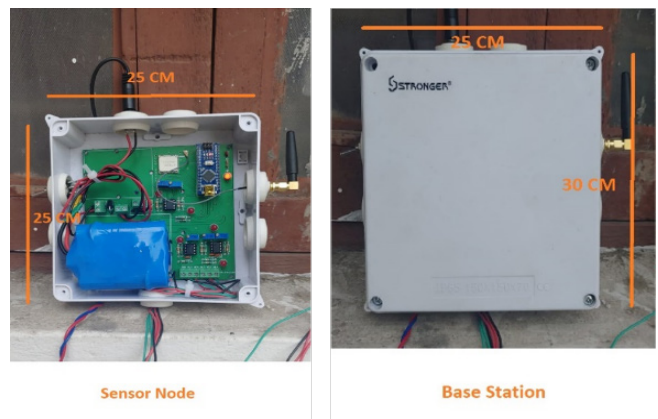
Figure 7: Final prototype featuring water sensing node (Left) and base station (Right)
