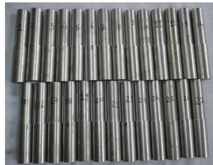
**Figure 3: Step making operation holding datum in chuck and 27 component after turning operation**
