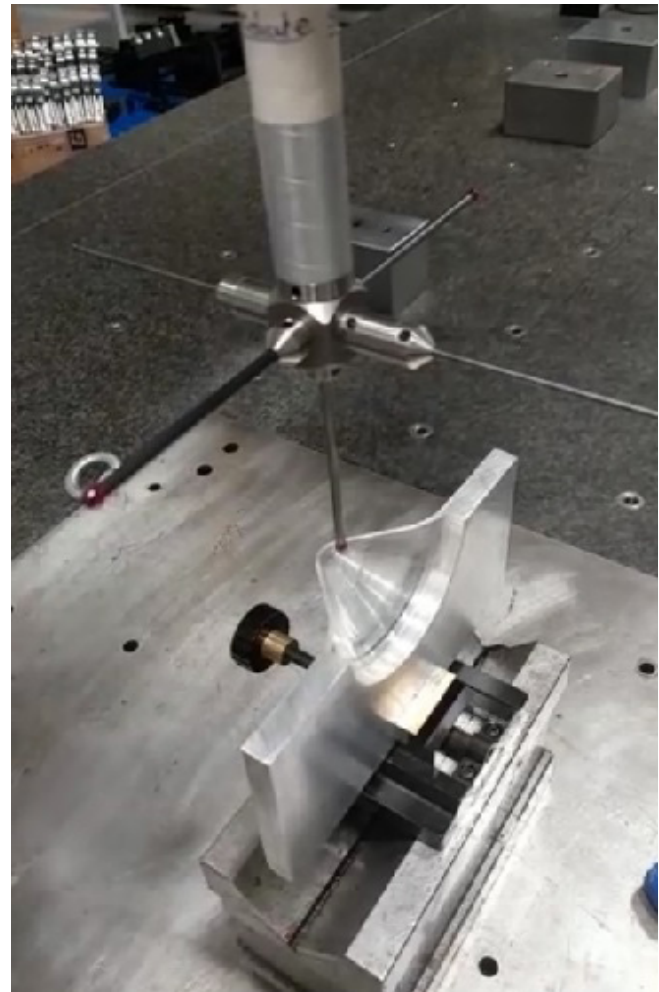
Figure 6: Thickness measurement using CMM
