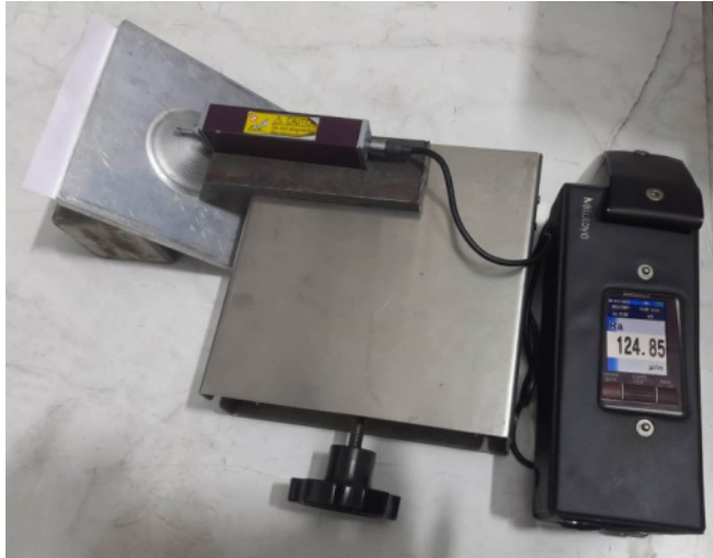
Figure 7: Surface tester measuring surface roughness
