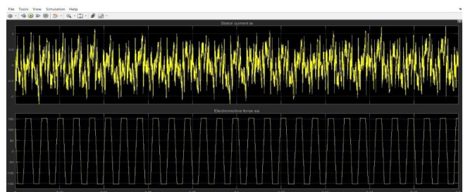
Figure 17: Stator current and EMF of the BLDC motor
