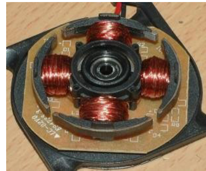
Figure 10: Construction of BLDC motor
